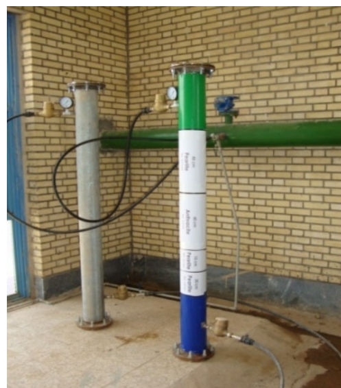
Fig. 2: Model of under pressure sand filters
